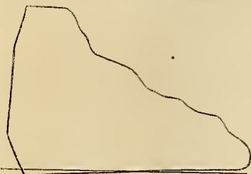
A. High-pressure—Bottom of Cylinder. Steam in Boiler ..... 115 Vacuum ..... 18 Revolutions ..... 49½
